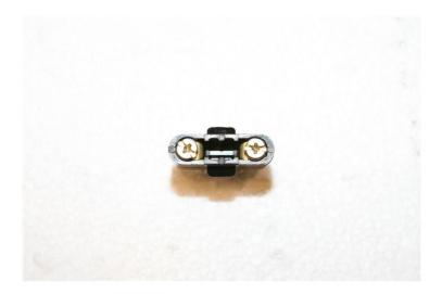
The 47K, 1 Watt resistors I got are the small power resistor type, and they are placed between the two screw terminals so that when you bend the leads they are in the tightening direction:
