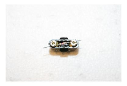
Once you bend the leads and tighten the screws down, it looks like this. Notice how the resistor sits down inside the body of the unit, tucked out of the way:
